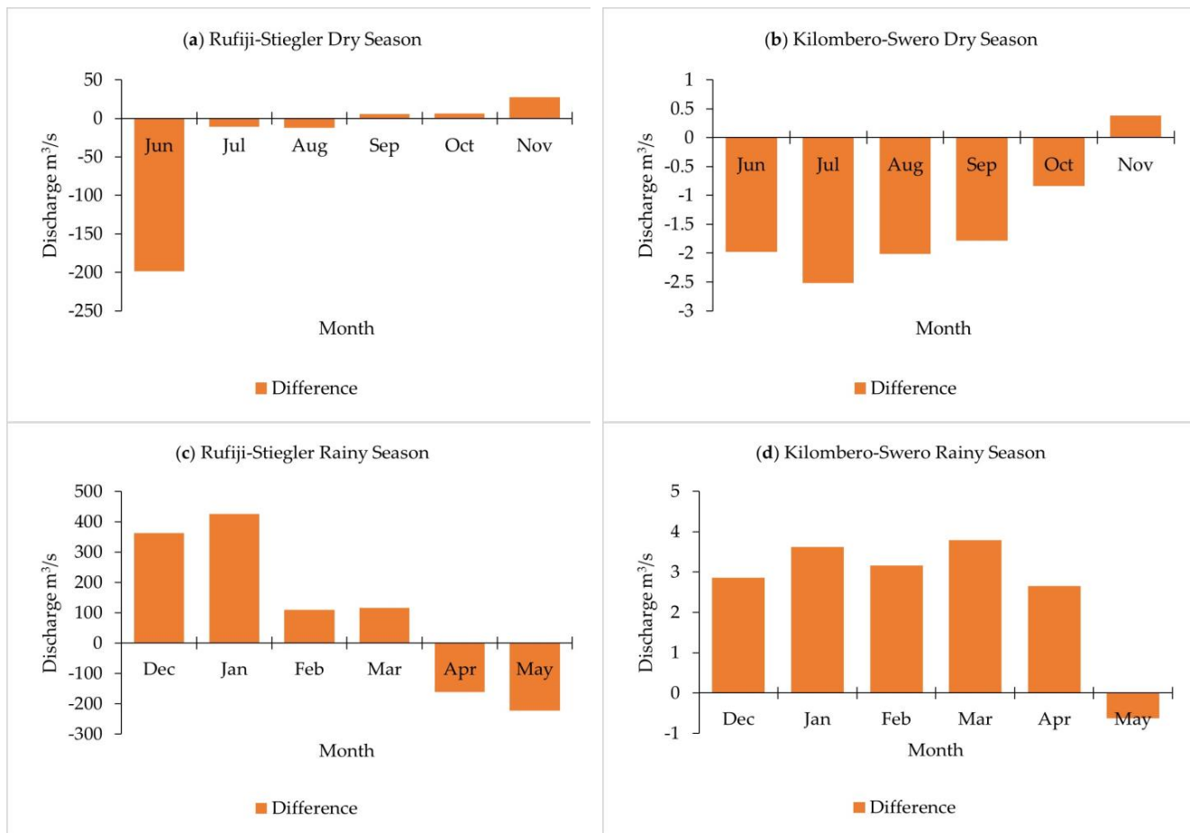
Figure 6. Comparison streamflow change between without and with-dam scenario for the years 2000 to 2022. (a,b) Dry season (June–November), (c,d) rainy season (December–May). Difference is equal to without-dam minus with-dam.
