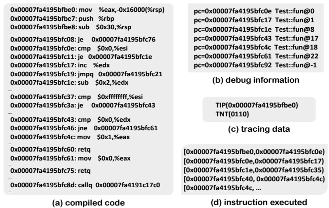
Figure 3. Flow reconstruction for JITed code: (a) compiled code for the program in Figure 2(a); (b) the debug information generated by compilation; (c) its hardware trace; and (d) the machine instructions executed.
