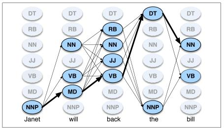
Figure 17.11 A sketch of the lattice for *Janet will back the bill*, showing the possible tags  $(q_i)$  for each word and highlighting the path corresponding to the correct tag sequence through the hidden states. States (parts of speech) which have a zero probability of generating a particular word according to the B matrix (such as the probability that a determiner DT will be realized as Janet) are greyed out.
