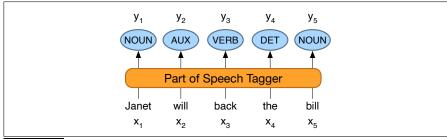
**Figure 17.3** The task of part-of-speech tagging: mapping from input words  $x_1, x_2, ..., x_n$  to output POS tags  $y_1, y_2, ..., y_n$ .
