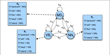
**Figure 17.9** An illustration of the two parts of an HMM representation: the *A* transition probabilities used to compute the prior probability, and the *B* observation likelihoods that are associated with each state, one likelihood for each possible observation word.
