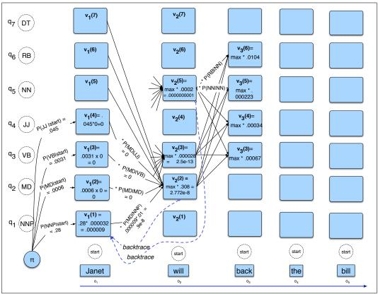
**Figure 17.14** The first few entries in the individual state columns for the Viterbi algorithm. Each cell keeps the probability of the best path so far and a pointer to the previous cell along that path. We have only filled out columns 1 and 2; to avoid clutter most cells with value 0 are left empty. The rest is left as an exercise for the reader. After the cells are filled in, backtracing from the *end* state, we should be able to reconstruct the correct state sequence NNP MD VB DT NN.
