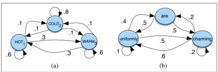
**Figure 17.8** A Markov chain for weather (a) and one for words (b), showing states and transitions. A start distribution  $\pi$  is required; setting  $\pi = [0.1, 0.7, 0.2]$  for (a) would mean a probability 0.7 of starting in state 2 (cold), probability 0.1 of starting in state 1 (hot), etc.
