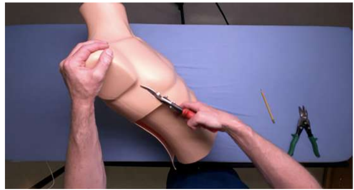
Figure 1. Cutting the dress form torso with tin snips to create the Yogaman chest tube trainer.
