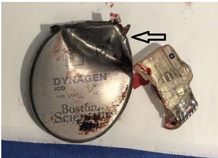
Image 3. Explanted automated implantable cardioverter defibrillator showing damage to the pulse generator (arrow) and separation of the header.
