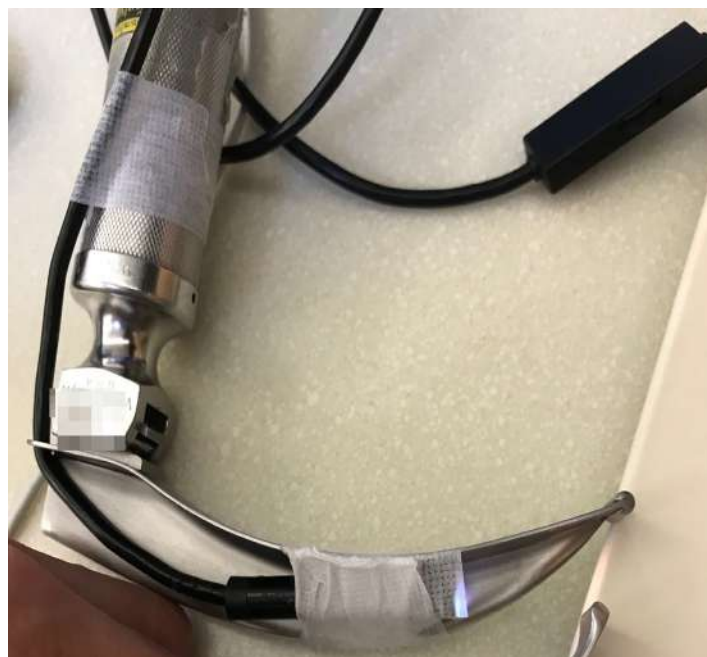
Figure. A low-cost videolaryngoscope created from the direct laryngoscope and a low-cost smartphone borescope.
