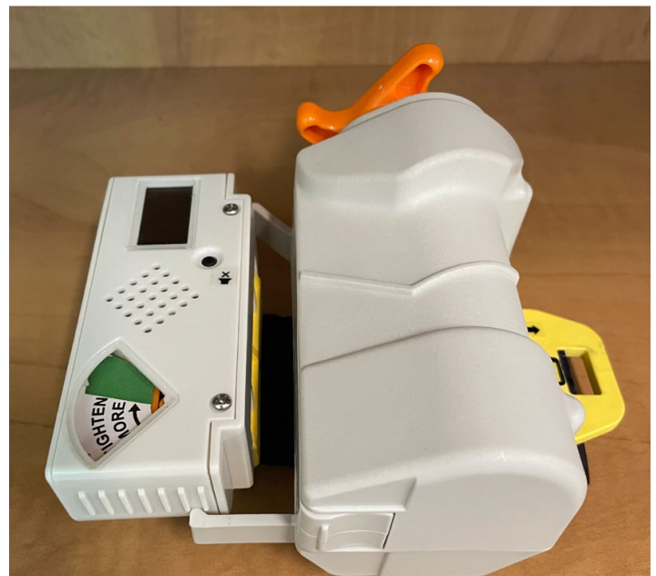
Figure 1. The LAVA TQ*: a user-intuitive tourniquet with a seatbelt design and audiovisual instructions.
