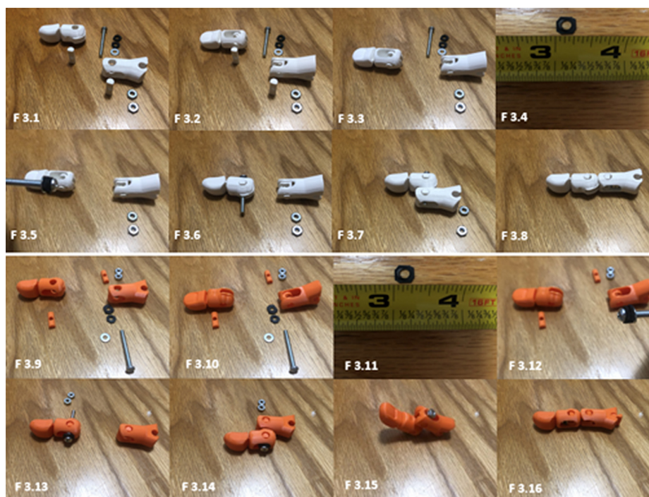
Figure 3. 3.1. Shows all component parts of the dorsally dislocated finger (lateral view). 3.2. Dorsal view. 3.3. Place pin and align the central opening with openings in the middle and proximal finger portions. 3.4. Modified neoprene washer cut \frac{1}{4} in x \frac{1}{4} in. 3.5. Load two neoprene washers and a machine screw nut. 3.6. Load the screw dorsally through the pin. 3.7. pass screw through pin in proximal phalanges as shown and attach screw nuts in this position. 3.8. Place in the reduced position to check resistance. 3.9. Shows all component parts of the volar dislocated finger (lateral view). 3.10. Dorsal view. 3.11. Modified neoprene washer cut \frac{1}{4} in x \frac{1}{4} . 3.12. Load two neoprene washers and machine screw nut. 3.13. Load the screw ventrally through the pin. 3.14. Pass screw through pin in proximal phalanges as shown and 3.15. attach screw nuts in this position. 3.16. Place in the reduced position to check resistance.
