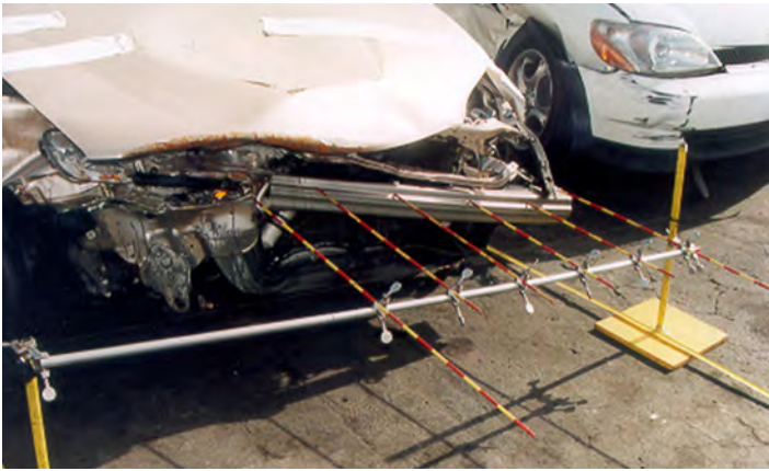
Figure 1. Frontal damage with measurement of vehicle deformation
