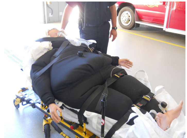
Figure. Mannequin in a water-filled bariatric suit on top of a tarp-style transportation device.
