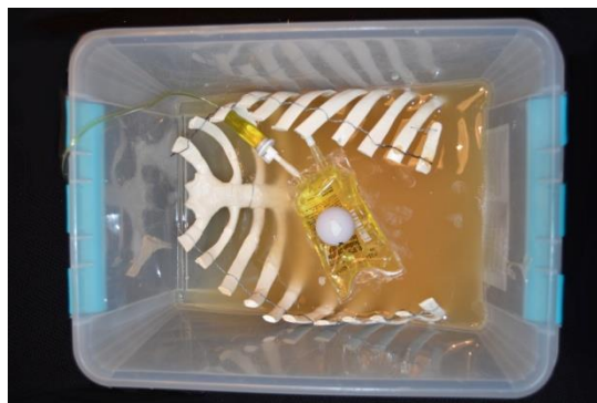
Figure 2. Melted gel wax is used to fill the artificial sternum, covering half of a ping pong ball that simulates the right ventricle.
