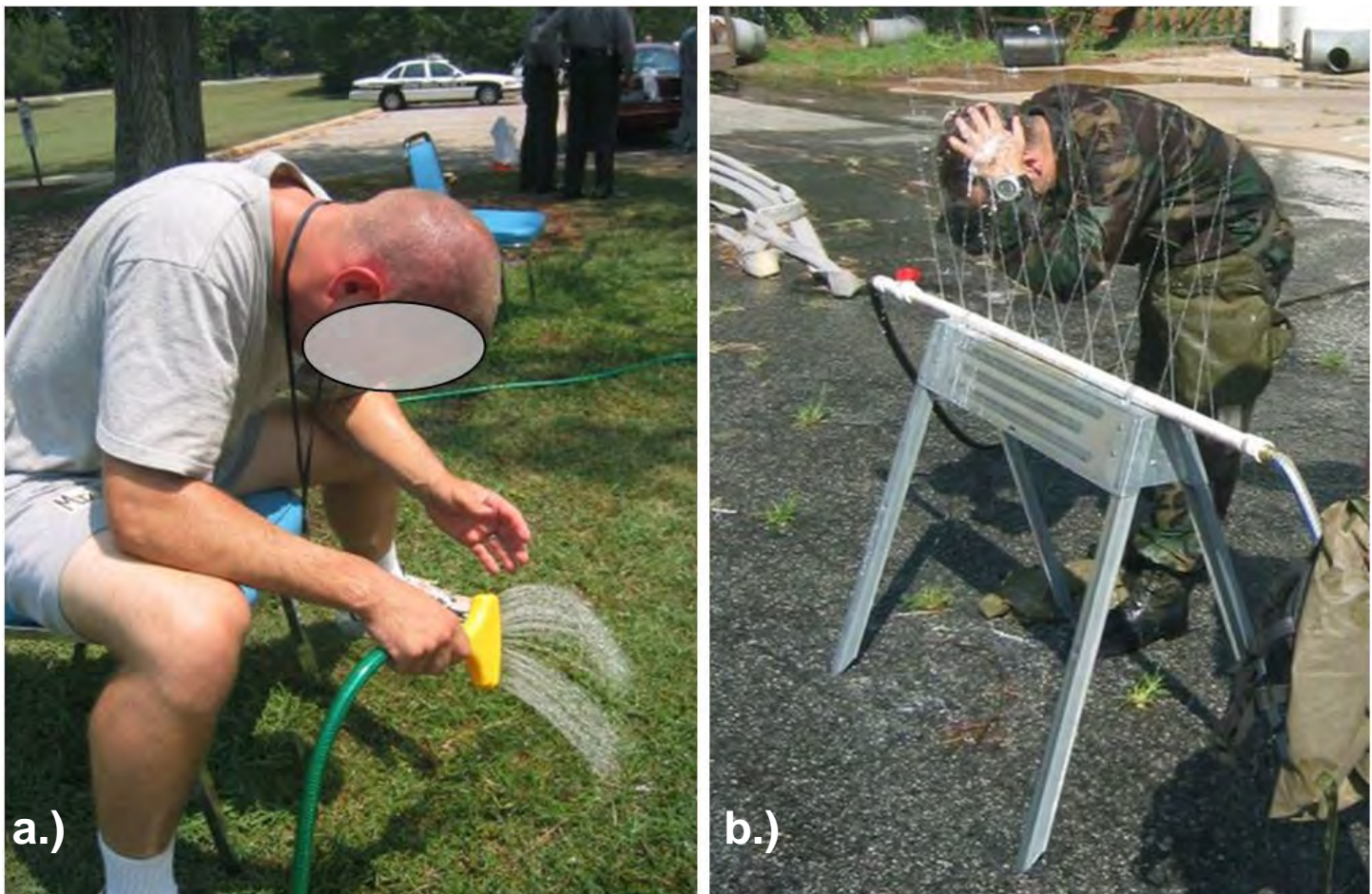
Figure 1. Irrigation technique and equipment for a) OC (pepper spray), and b) CS (tear gas).
