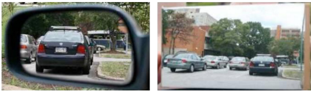
Fig. 6. Left image is from a flat driver-side mirror, and right one is from a freeform mirror [165].
