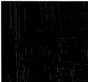
Figure 2.1: The PMF algorithm applied to our test stereo pair presented in figure B.1. Intensity of edges proportional to disparity.
