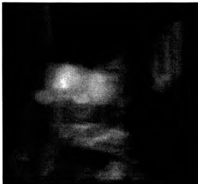
Figure 8.13: Intensity disparity image produced from figure B.1 using a single horizontally oriented 2-D filter as in figure 8.12.
