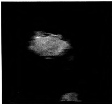
Figure 8.9: Intensity disparity image produced from figure B.1. 12 orientationally selective filters with aspect ratio 1:1 were used tuned to 0.25 cpp. Images compressed to 16x16 at the lowest resolution.
