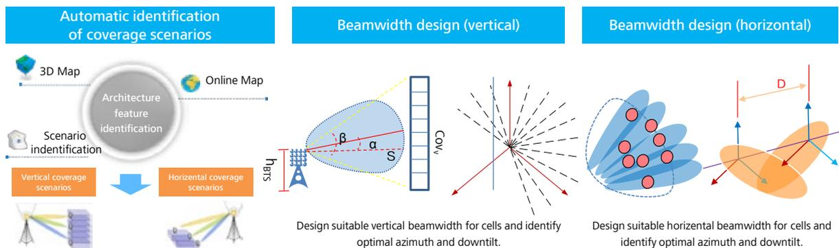
Figure 2-9 ACP functions for precise RF parameter planning
