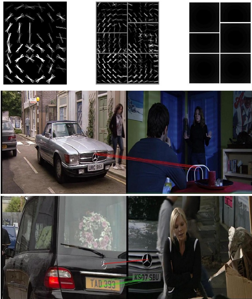
Fig. 3. First row: DPM model of Mercedes logo. Second row: shared word matching after geometric verification. Third row: Reranking combining BOW model and DPM object detection algorithm. (Programme material copyrighted by BBC.)
