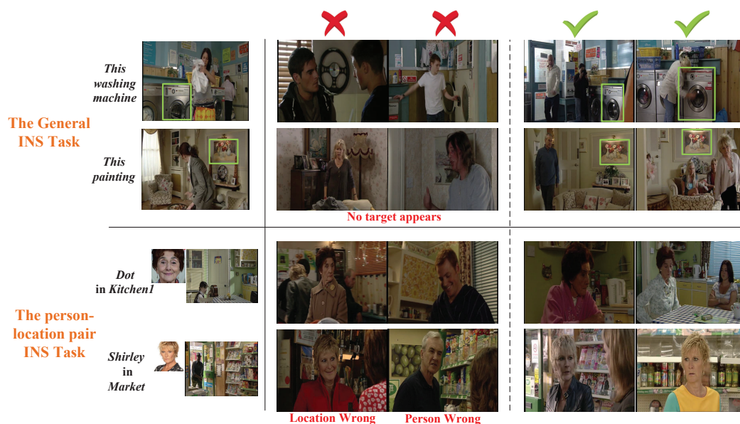
Fig. 1: Examples for general INS task (top) and person-location pair INS task (bottom). For the general INS task, the system only needs to search out corresponding shots with certain objects, such as this washing machine and the painting . If the certain object appears in the shot, the shot is the positive one. For person-location pair INS task, the system requires to search out the target person in the right location at the same time, such as “ Dot in Kitchen1 ” and “ Shirley in Market ”. If target person or target location does not appear simultaneously, the shot will be considered as a negative one. The examples are selected from the TV series Eastenders . Programme material copyrighted by BBC.
