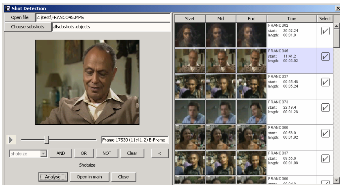
Figure 4: Screenshot of the graphical user interface for the retrieval component. The retrieval list on the right side shows the result for the feature shot size = 30%.
