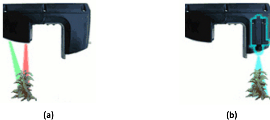
Figure 33: Operating principle of the Weedseeker. (a) Detection of green weeds thanks to their reflectance. (b) Spraying of herbicides only on green weeds (source: http://www.avidorhigh tech.com/html/weedseeker.html ).
