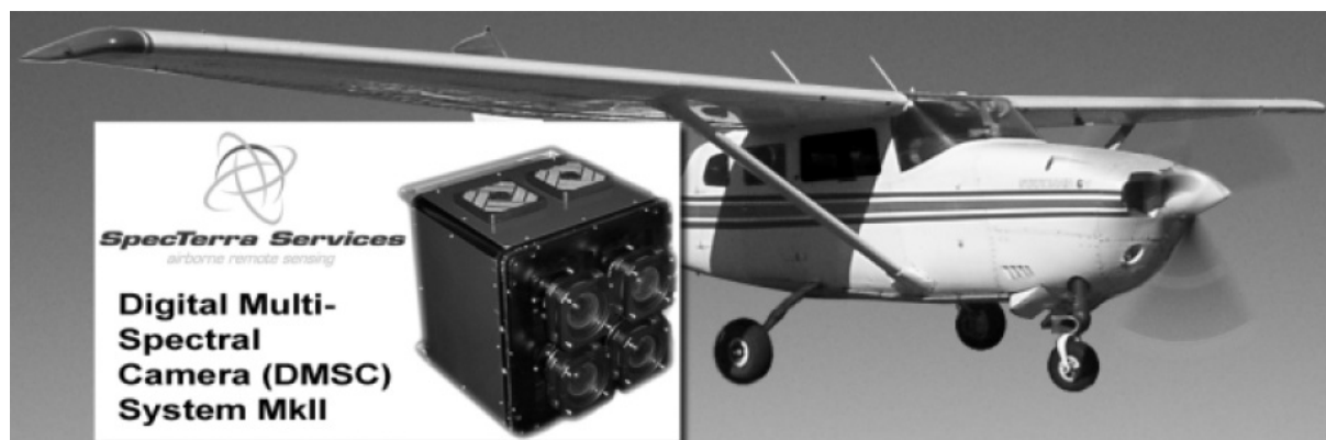
Figure 3: Cameras mounted underneath the aircraft with a computer on board which collects the data (source: Proffitt, 2005).
