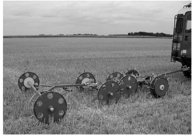
Figure 28: Resistivimeter pulled: Multidepth Continuous Electrical Profiling (MUCEP) (source: Samouëlian et Al., 2005).
