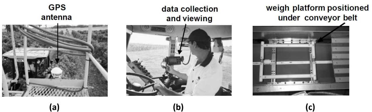
Figure 10: Equipment required to record yield. (a) GPS antenna mounted on the harvester. (b) Computer in the tractor to collect and to view data. (c) Gravimetric yield-monitoring system with a weigh platform positioned under the conveyor belt (source: Proffitt, 2005).
