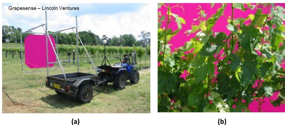
Figure 17: (a) Pink screen mounted on a four-wheel motorbike to make ground-based measurements. (b) Photograph of a row taken with the pink screen placed behind the row (source: Tuohy, 2005).
