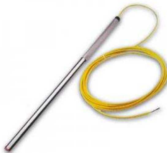
Figure 34: TDR sensor ( source: http://www.envcoglobal.com ).
