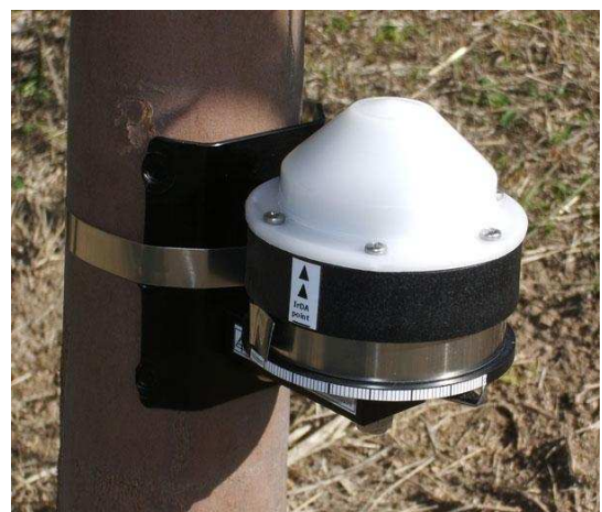
Figure 23: Dendrometer (source : http://www.ictinternational.com.au ).
