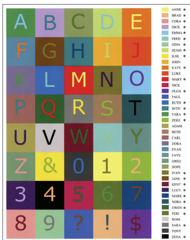
Figure 12 Sheet used to test people’s ability to recognise colours under the influence of simultaneous contrast
