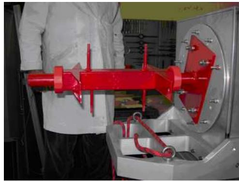
Fig. 4. Setup used for flexure measurements of the IFS bench - 1.
