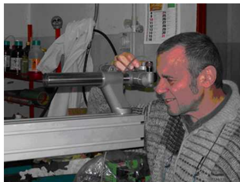
Fig. 5. Setup used for flexure measurements of the IFS bench - 2.
