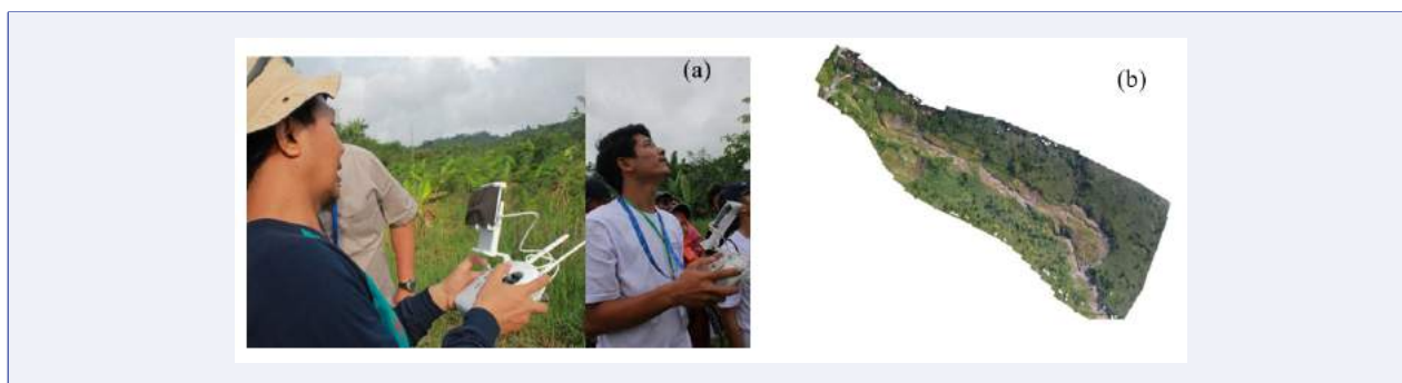
FIGURE 5. Field data acquisition (a) and orthophoto map derived from UAV data (reproduced with permission of Sutrisno et al., 2017 ) (b).
