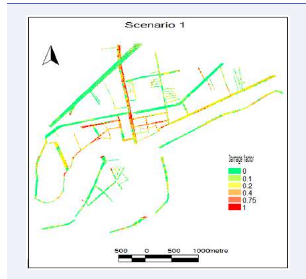
FIGURE 8. Flood risk map for urban roads under SCE_1 in Samut Sakhon city.
