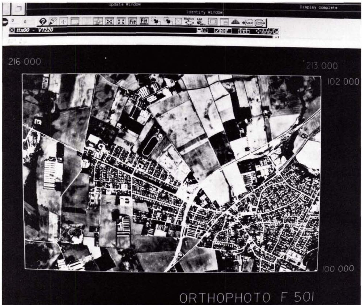
Figure 4. Digitally produced orthophoto of a 2- by 3-km area in Denmark. Geometric resolution: 0.4 m by 0.4 m on the ground.
