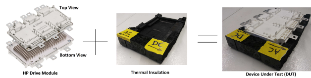
Figure 13: The DUT with the Thermal Package for the Calorimetric Test Bench
