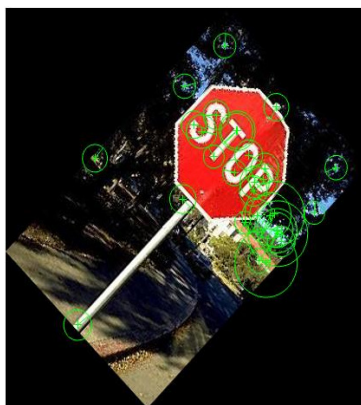
Figure 3: SURF Features Detection in rotated (30°) and scaled (1.5) image
