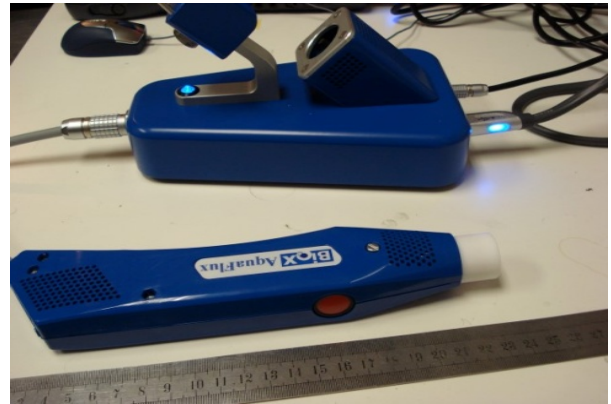
Figure 3. AquaFlux probe measured by a ruler
