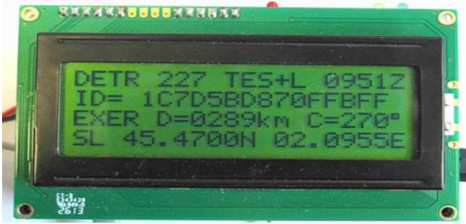
Figure 5. The GPS position transmitted by the beacon
