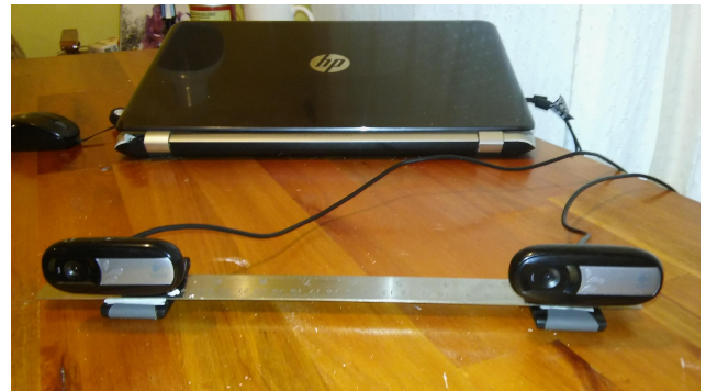
Figure 7: A notebook connected to two regular cameras mounted in a platform with known distance and orientation.
