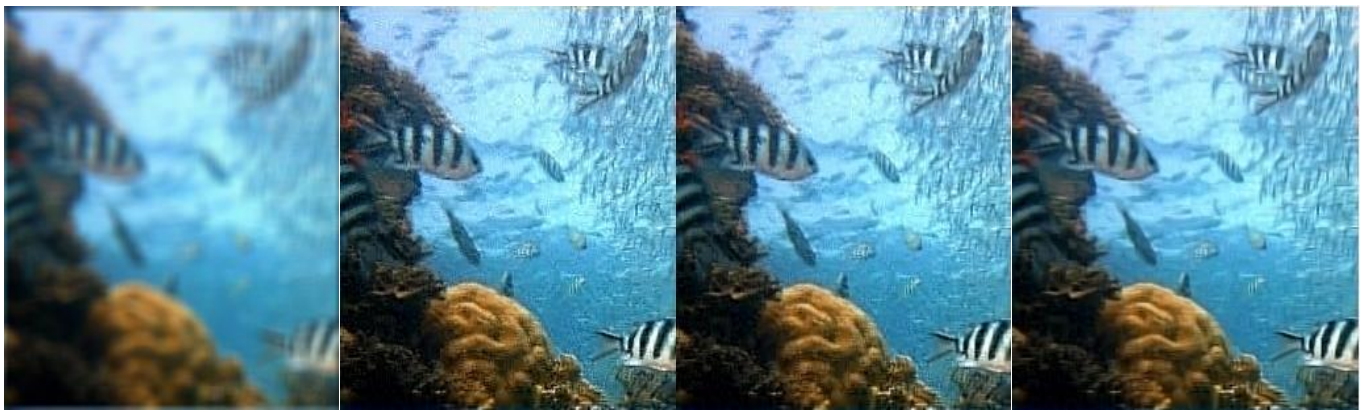
(i) (ii) (iii) (iv) Figure 3: Underwater Turbidity Removal. (i)Blurred picture (ii) ASDS (iii) ASDS using AR (iv) ASDS using AR and NL
