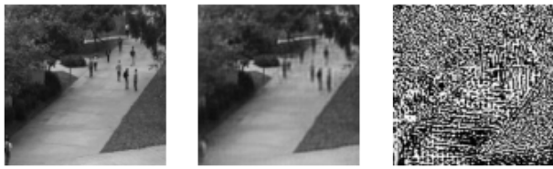
(a) Input frame on the left, reconstructed frame on the middle, and the difference between input and reconstructed frame on the right
