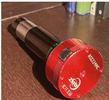
Image 2: The author's CMOS camera, a ZWO ASI224MC with a 3x Tele Vue Barlow
