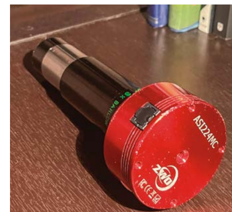
Image 2: The author's CMOS camera, a ZWO ASI224MC with a 3× Tele Vue Barlow
