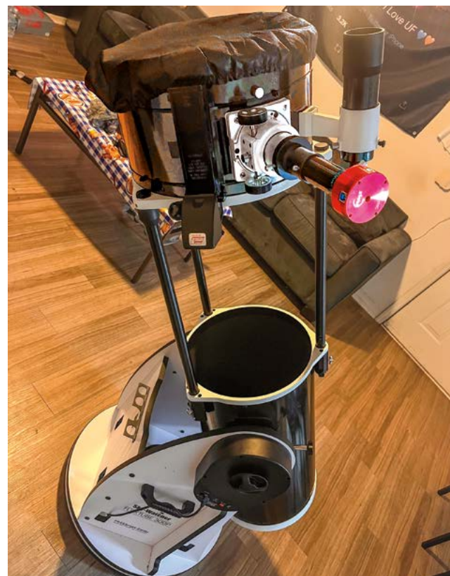
Image 5: The author's Sky-Watcher 300P Flextube Dobsonian with a ZWO ASI224MC CMOS camera
