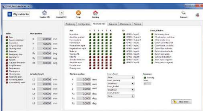
Window allowing the user to get an overview of the hexapod current state.
