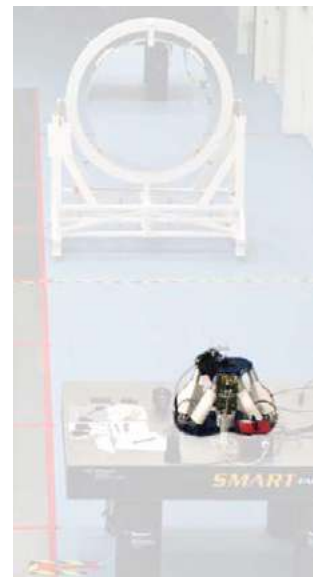
The BREVA hexapod is part of the ESA Star Tiger-2 test set-up to simulate a way to eclipse the Sun in space with two satellites flying in tight formation.
