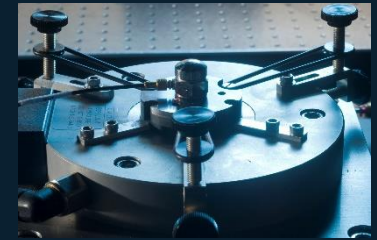
Measurement calibration bench for accelerometer calibration by primary means
