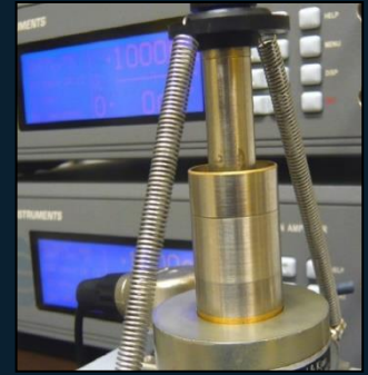
Measurement standards for sound pressure based on reciprocity calibration of measurement microphones
