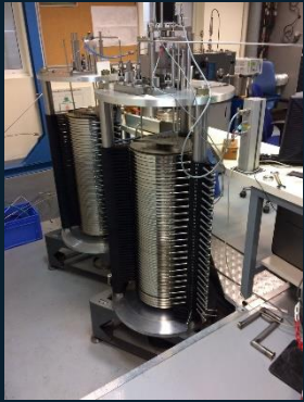
Measurement standards for static pressure based on the pressure balance
