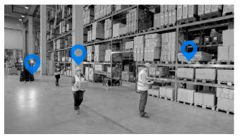
Using a Bluetooth RTLS solution, key resources in a warehouse, like pallets, forklifts and workers, can be easily located and tracked.
