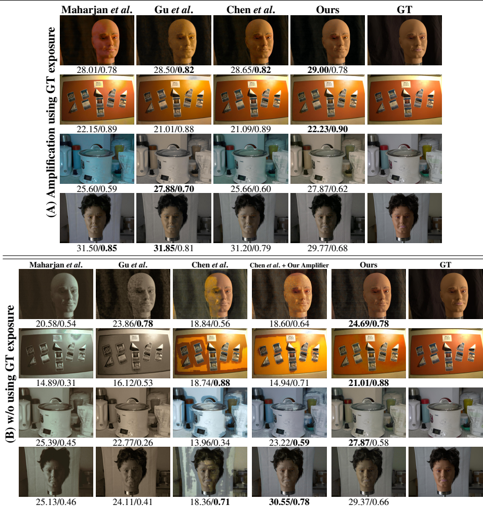
Figure 4: [View with good screen brightness] Performance comparison of the proposed LLPackNet with state-of-the-art algorithms corresponding to Table 1. (A): All the methods work well with GT exposure. (B): But in a realistic scenario, where exact GT exposure may not be available during inference, only the proposed LLPackNet gives proper restoration.
