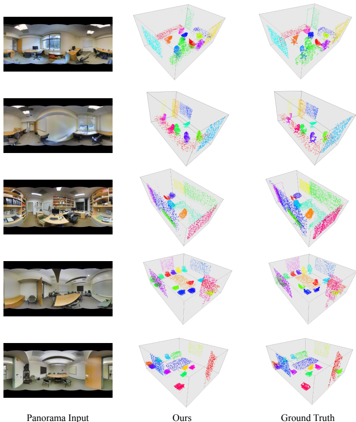
Figure 5: Qualitative results for 3D semantic scene reconstruction. Given a single panorama image, our method (end-to-end) reconstructs the 3D indoor semantic scene point cloud.
