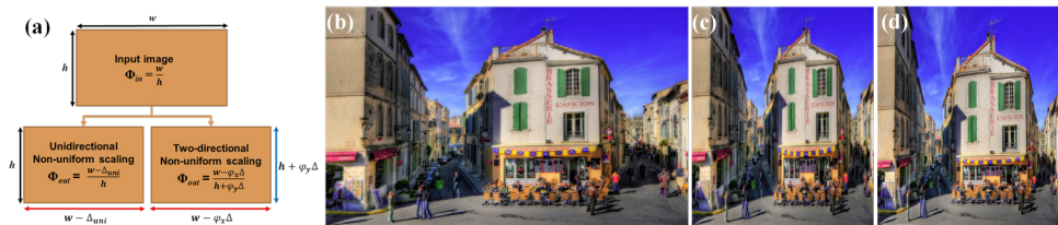
Figure 3: Difference of proposed approach compared with the unidirectional non-uniform scaling. (a) Conceptual example of unidirectional and two-directional non-uniform scaling, (b) Input image (1024x622, \Phi_{in} \doteq 1.64 ), (c) Cycle-IR [20] (512x622, \Phi_{out} \doteq 0.82 ), (d) Proposed approach (720x875, \Phi_{out} \doteq 0.82 ).
