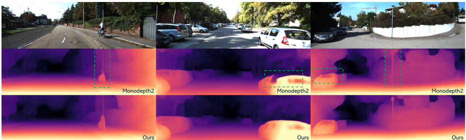
Figure 2: Depth estimation on three sample images. The second row shows the estimated depth maps by Monodepth2 [9] and the third row shows the depth maps by our proposed X-Distill approach. It can be seen that our method provides more accurate depth estimation. The green boxes indicate sample regions where our method considerably improves the estimation quality.
