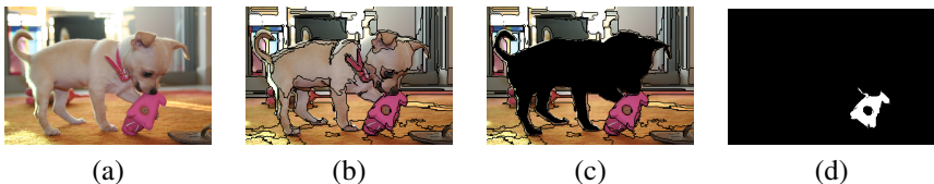
Figure 2: Step-by-step breakdown of pseudo-mask generation for self-supervision. (a) Input query image. (b) Generate superpixels in the query image. (c) Remove superpixels that coincide with the original class ground truth. (d) Randomly sample superpixel with high corresponding feature activation, and convert it into a binary mask.
