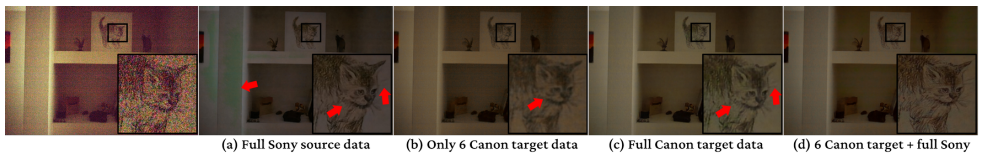
Figure 1: Qualitative comparison between different methods with an input to the model from the Canon dataset (left-most). The models are: LSID trained on (a) full 161 Sony source images, (b) only 6 Canon images, and (c) full Canon dataset. (d) 6 Canon images and 161 Sony images with proposed few-shot domain adaptation method (discussed in section 3).
