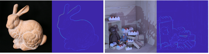
Figure 5: Estimated depth edge confidence \lambda_s . The bi-directional diffusion process allows us to identify depth edges by considering the mean gradient at each pixel across the backward-forward pass. Texture edge gradient remains low in both passes. For depth edges, the gradient is higher in one pass. For depth edges that are not meant to be sharp, the change in depth around that region from the bi-directional solve is small, and picking either offset leads to low error.
