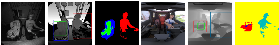
Figure 1: From left to right Real IR image, real depth image with 2D bounding box annotation, real image segmentation mask, synthetic RGB image, synthetic depth image with 2D bounding box annotation, synthetic image segmentation mask.
