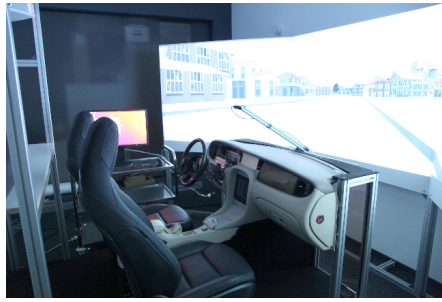
Figure 2: Our data capturing setup equipped with a wide-angle projection system, car front seats and a Kinect Azure camera in the front.
