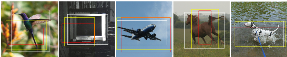
Figure 4: Visualization of the bounding box refinement during training. The red boxes denote the noisy annotations in the training dataset with the noisy parameters of N_{Label} = 40\% and N_{BBox} = 40\% . The correction results of the first step are shown in yellow boxes, whereas the final correction results are shown in white boxes.
