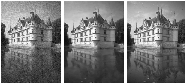
Figure 1: Left: Noisy image f with \sigma = 25 ; Middle: solution of (7), TNRD(f) , with u(t=0) = f , PSNR=29.64, SSIM=0.8496, Right: solution of (5) with \lambda = 0 , an oracle \kappa_{\mathcal{F}} = \kappa(a) and f_{in} = TNRD(f) , PSNR=33.69, SSIM=0.9289.
