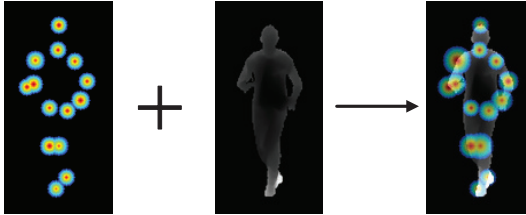
Figure 3: The depth with ad-pose is synthesized by the keypoint heatmap and the depth map.
