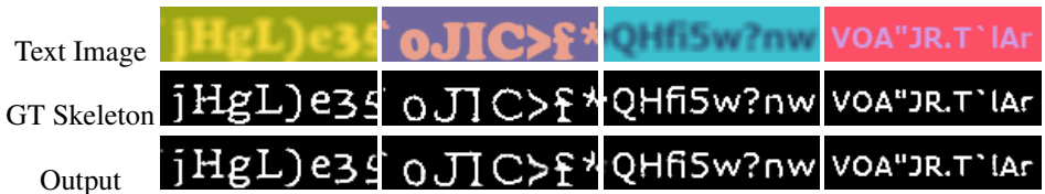
Figure 3: Examples of generated supervised data for training the skeletonization network. The top row shows synthetic text images, the middle row shows ground truth skeleton images, and the bottom row shows outputs of the trained skeletonization network.
