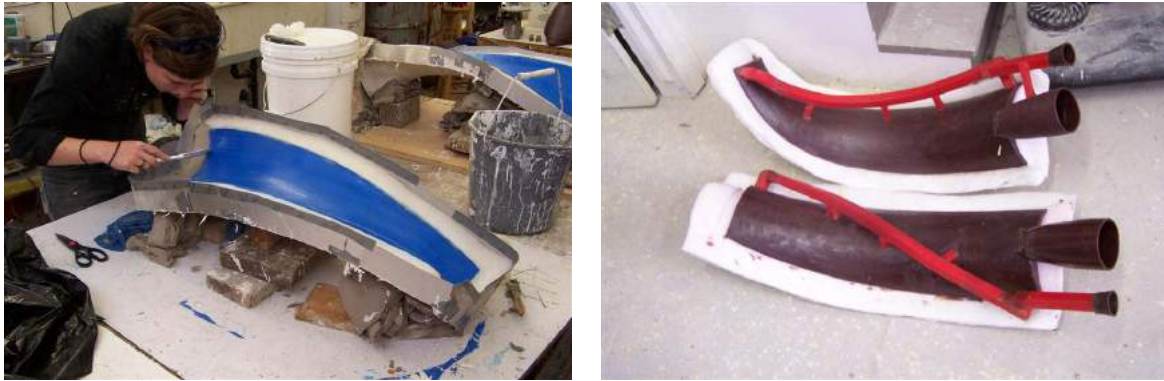
Fig. 12: (a) One third of the larger master segment used to form a mold; (b) wax copies of this sub-segment with sprues.
