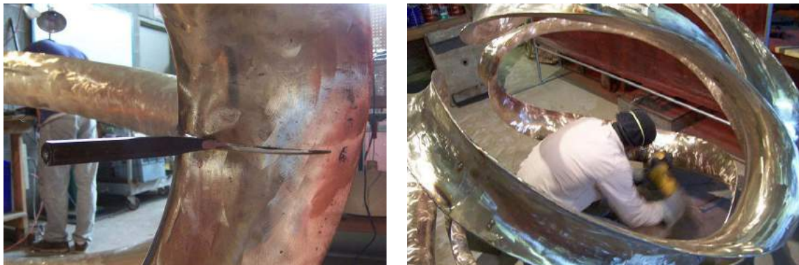
Fig. 15: (a) Adjusting the overall shape of Pax Mundi II by fine-tuning some of the bends; (b) grinding and polishing.
