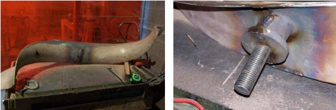
Fig. 14: (a) Two of the individually cast pieces welded together; (b) the support point for Pax Mundi 2 .
