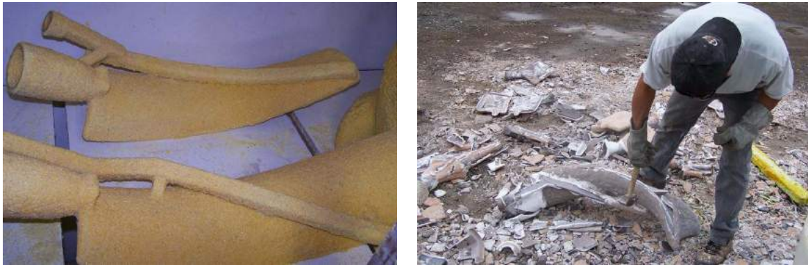
Fig. 13: (a) Slurry shell around wax copies; (b) removing the plaster shell after the casting process.
