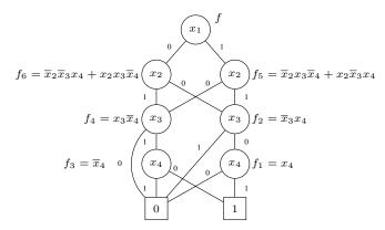
Figure 1: Decision diagram representing the Boolean function  $f = \bar{x}_1 \bar{x}_2 \bar{x}_3 x_4 + \bar{x}_1 x_2 x_3 \bar{x}_4 + x_1 \bar{x}_2 x_3 \bar{x}_4 + x_1 x_2 \bar{x}_3 x_4$
