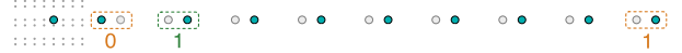
Fig. 6: The 1 st excited state of the BDL wire from Fig. 3a is transparent . The perturber on the left indicates a logic 1 input, which is inverted twice, leading to a correct output on the right.
