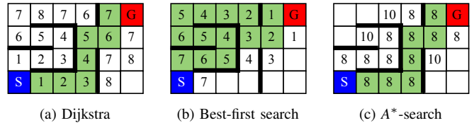
Fig. 3: Application of three different search algorithms to find a path (green) through a maze from start tile S (blue) to goal tile G (red).
