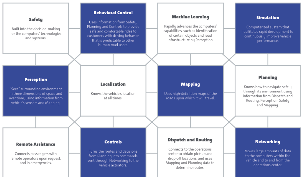
Figure 5. The building blocks of the automated driving system (General Motors 2018)
