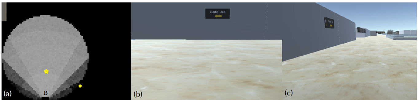
Figure 6: (a) Visualization of the probability of perceiving the information from Sign B. The yellow star and circle represent two locations where information is high and low with respect to sign B (b) First person view from the yellow star where information is high with respect to sign B (c) First person view from the yellow circle where information is low with respect to sign B.
