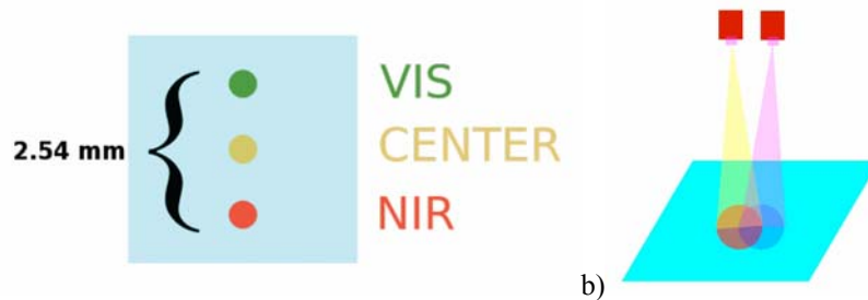
Fig. 2. Illustration of MISI's focal plane (a). VIS and NIR channels are off the center axis. This results in a slight misregistration between the VIS and NIR channels shown in (b).
